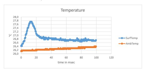
During the first pass the peak temperature was 27.8 °C on the surface.
