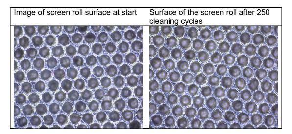
The images show that the JetCleaning AL1500 cleaning laser is not damaging the cell walls!
