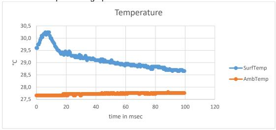
There is some increase in the ambient temperature and the maximum measured temperature on the surface is 30.3 °C.
