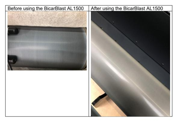
The BicarBlast AL1500 reduced their screen roll cleaning cost from about 23 euro for conventional cleaning to 2 euro for applying the BicarBlast AL1500 cleaning laser per screen roll sleeve per cleaning cycle.
