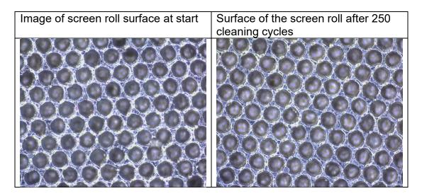
The images show that the BicarBlast AL1500 cleaning laser is not damaging the cell walls!
