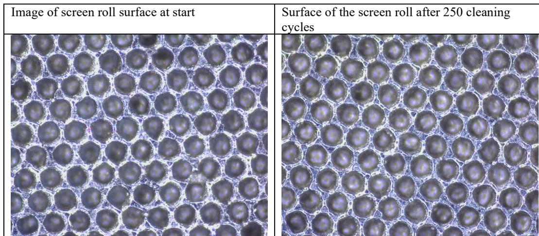
*The images show that the BicarBlast AL1500 cleaning laser is not damaging the cell walls (image: Technology Coaching BvbA)*
