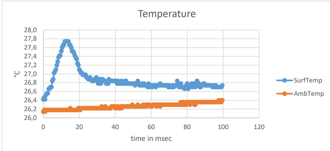
During the first pass the peak temperature was 27.8 °C on the surface.
