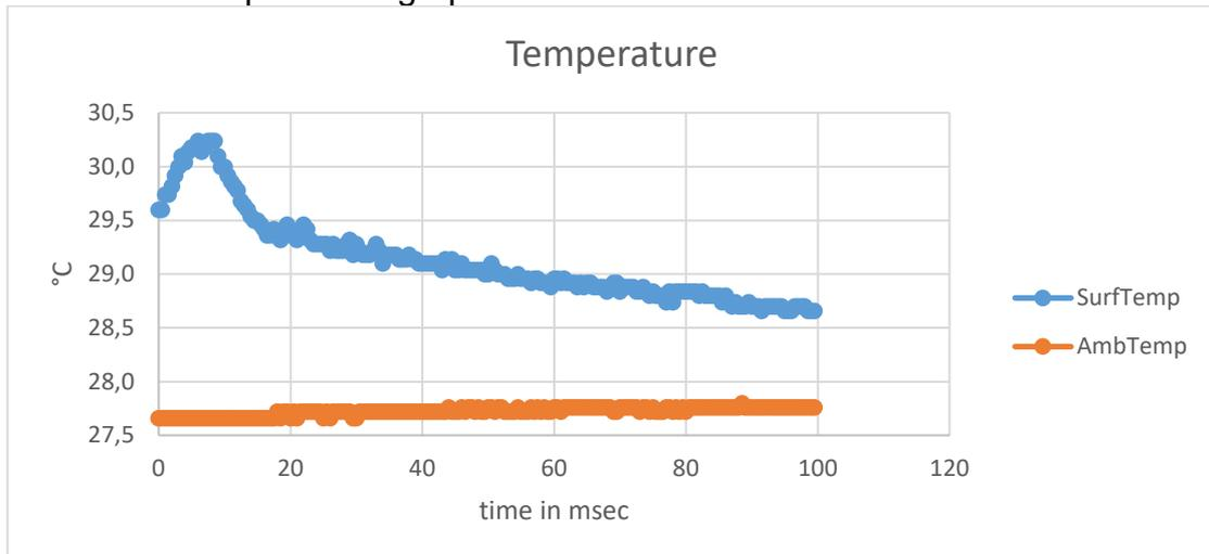
There is some increase in the ambient temperature and the maximum measured temperature on the surface is 30.3 °C.
