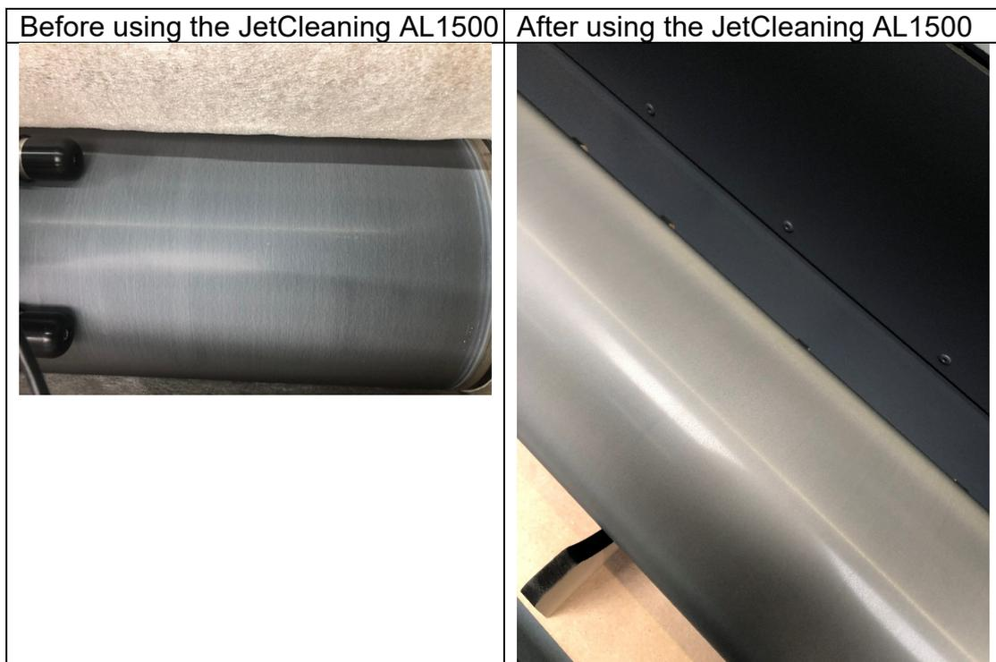
The JetCleaning AL1500 reduced their screen roll cleaning cost from about 23 euro for conventional cleaning to 2 euro for applying the JetCleaning AL1500 cleaning laser per screen roll sleeve per cleaning cycle.
