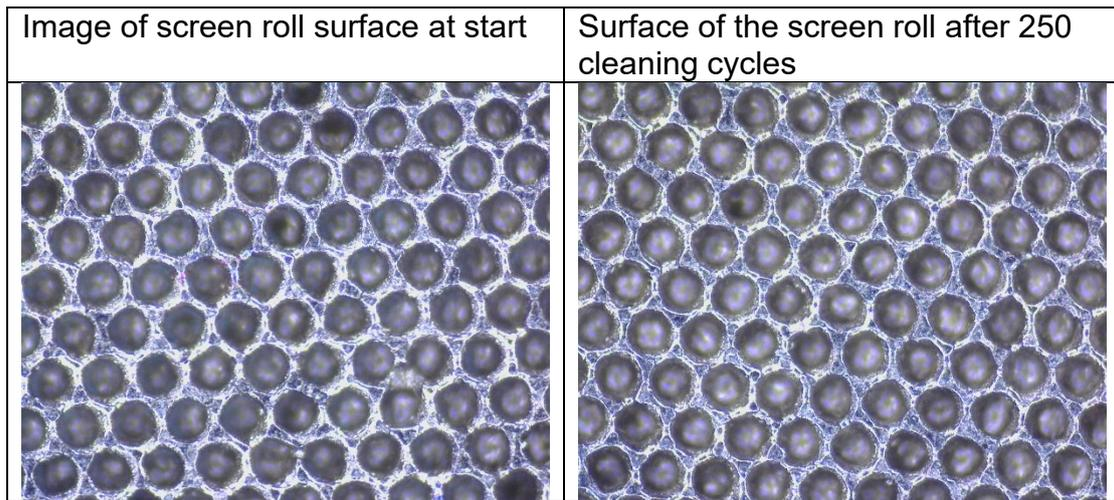
The images show that the JetCleaning AL1500 cleaning laser is not damaging the cell walls!
