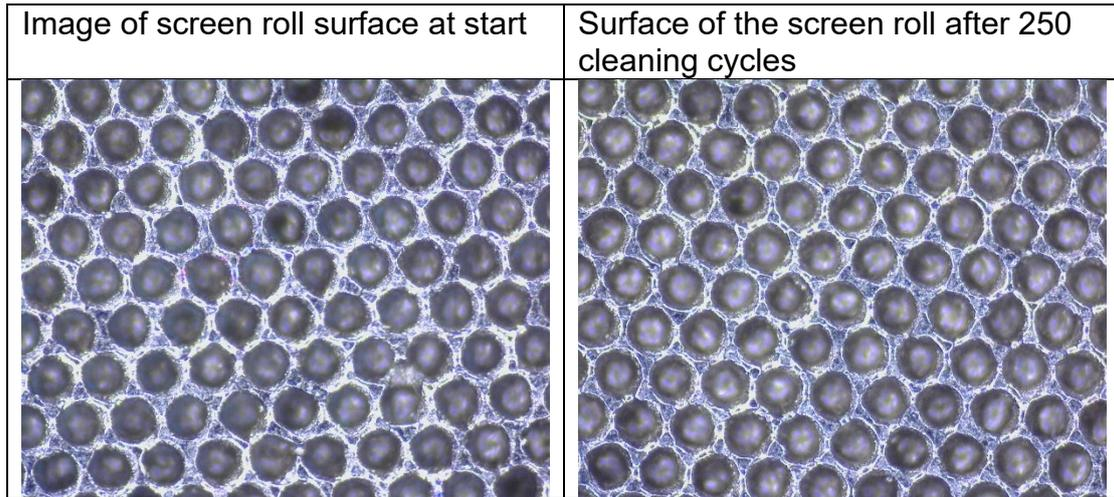
The images show that the BicarBlast AL1500 cleaning laser is not damaging the cell walls!
