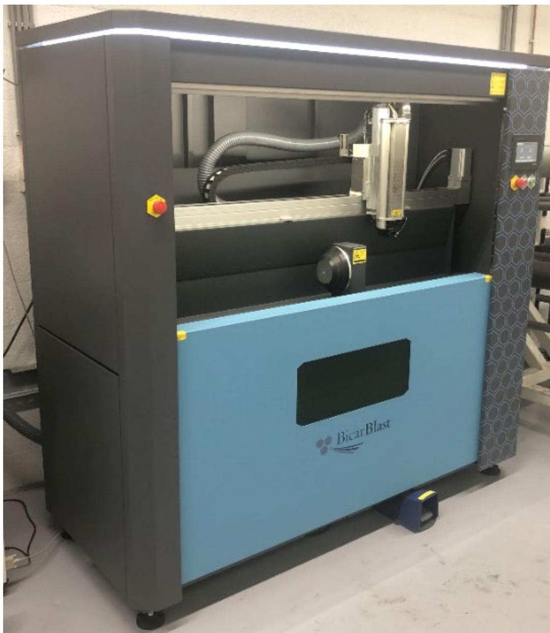
BicarBlast developed the AL1500 a laser for cleaning screen rolls (anilox rolls) and screen roll sleeves that is not damaging the surface of the screen roll.
